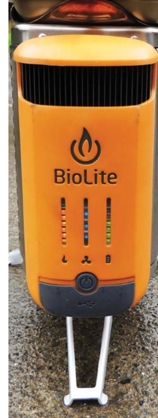
The LED lights from left to right indicate heat/power, fan speed and battery charge.
